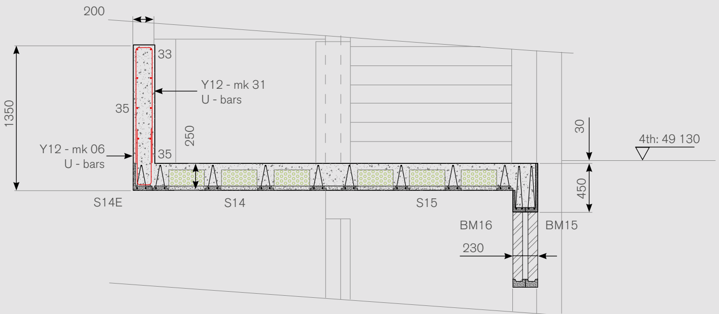
This sketch shows the integration of the Cobute precast stair with the in-situ parapet.
